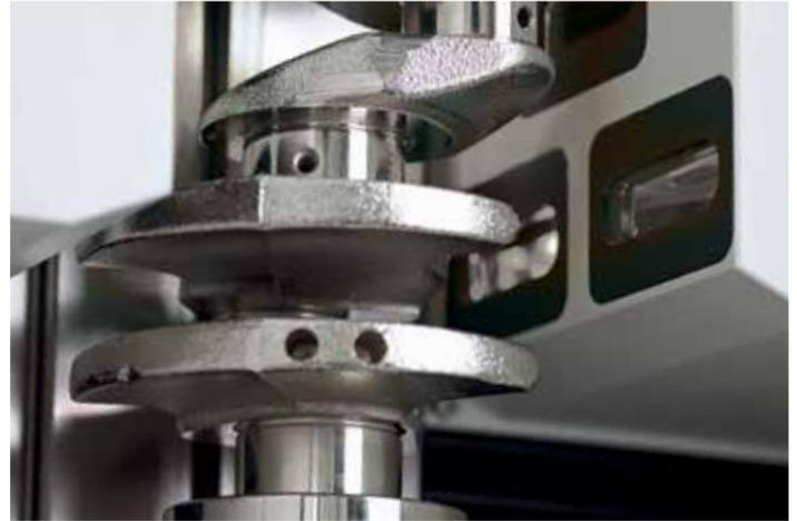
Measuring crank shafts with an Opticline C1023-75AE
