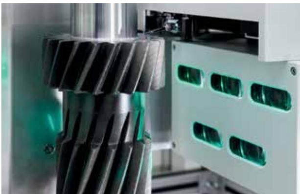
Optional tactile probing system for lengths and axial run-out
