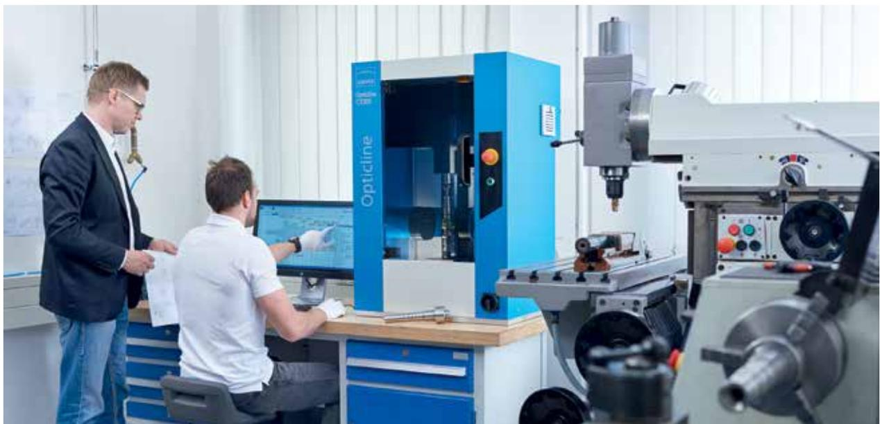
Opticline CS305 for cost-effective measurement of turned parts up to 300 mm in length
