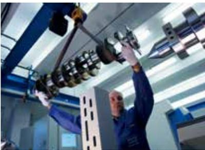
Use in production, loading a crank shaft with operator self-inspection
