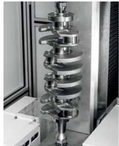
Opticline CA618-AE for measuring crank shafts
