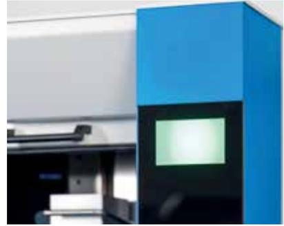
Results view visible from a distance for OK, NOK, warning limit and errors
